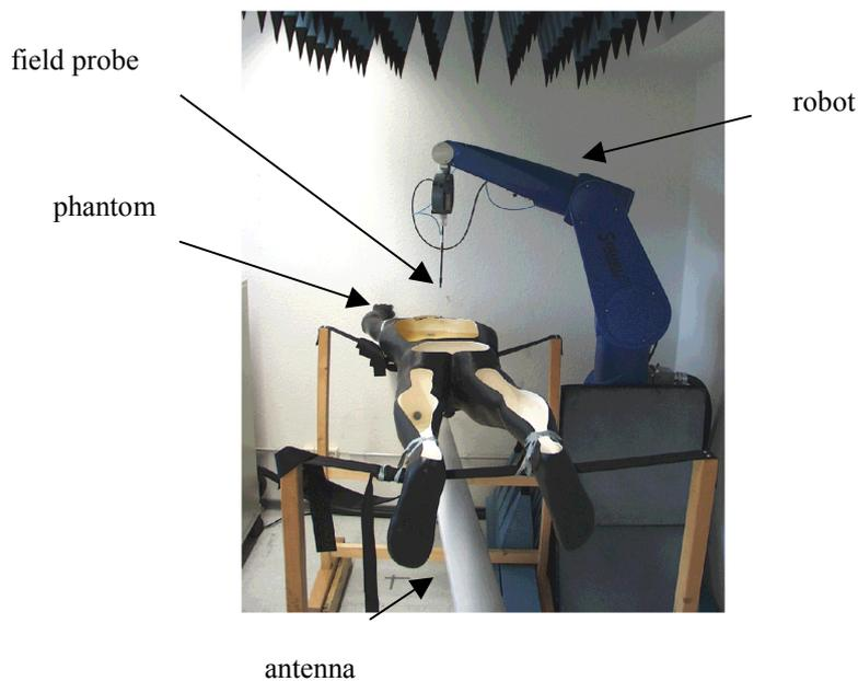
Fig. 2: Arrangement of the base station antenna, the phantom and the field probe for the analysis of the specific absorption rate SAR.
