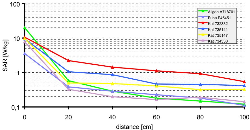
Fig. 3: Maximum localised SAR values (averaged over 10 g tissue) in the trunk of the phantom as a function of the distance  $d$  between phantom and base station antenna.
