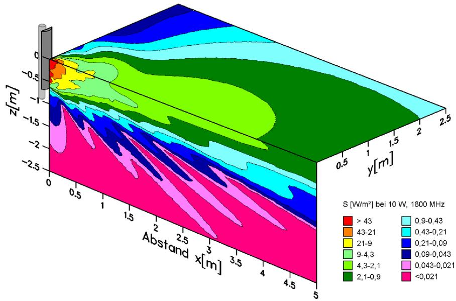
Fig. 1: Near field calculation of a 65°/18 dBi antenna at 1800 MHz with 10 W output power.
