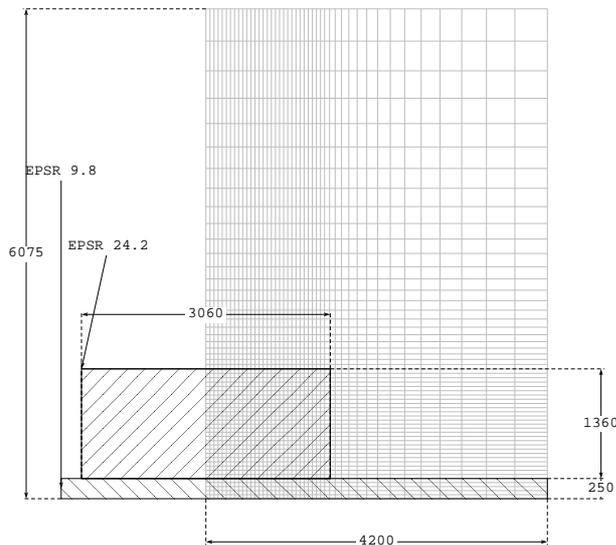
Fig. 1. Dielectric Resonator ( $\epsilon_r = 24.2$ ) on an  $\text{Al}_2\text{O}_3$  substrate.
