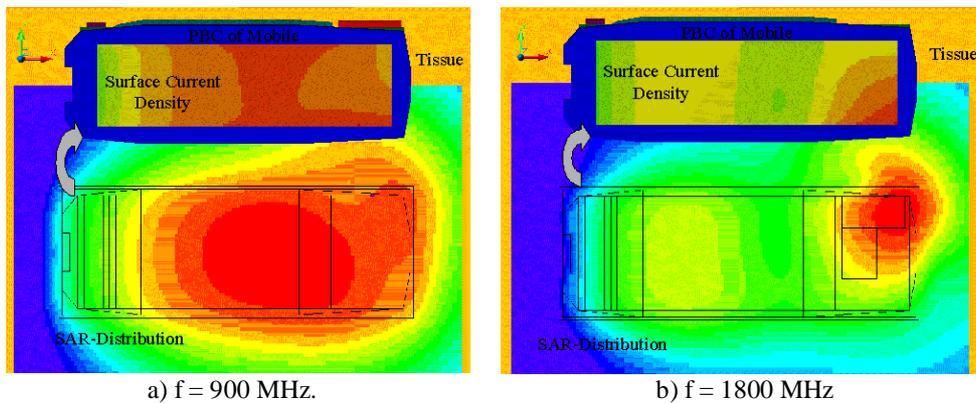
Fig. 2: Relation of the Surface Current Distribution on the PCB and the SAR induced in the flat-phantom: Length of mobile 110 mm.
