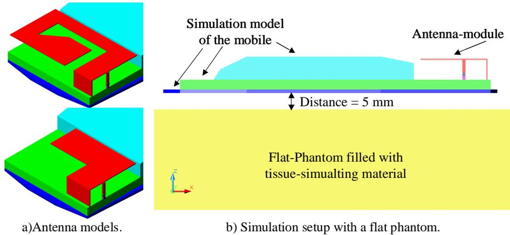
Fig. 1: Mobile placed in 5 mm distance above a flat-phantom.
