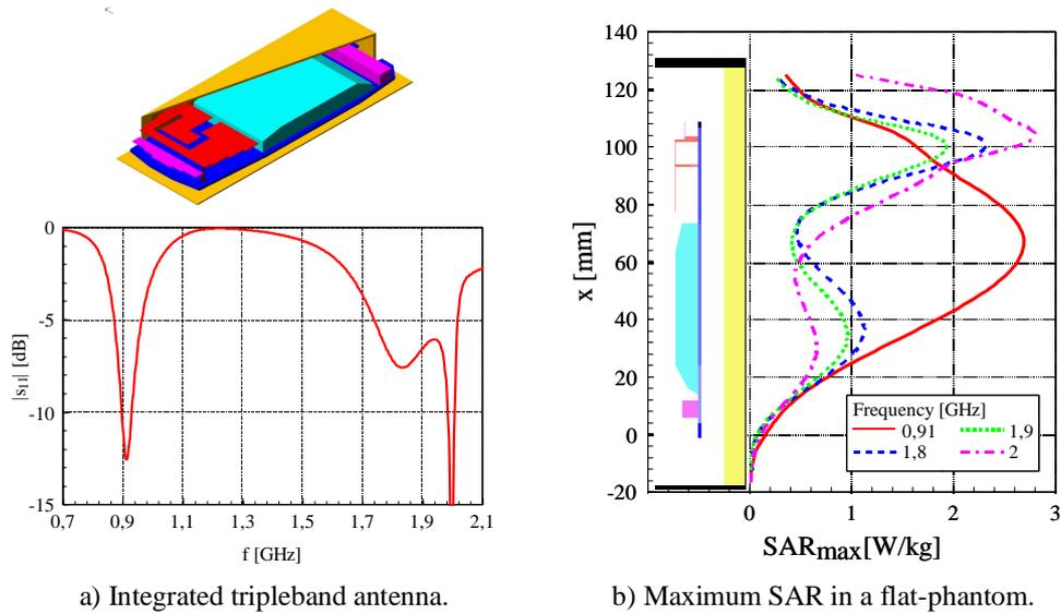
Fig. 4: An integrated tripleband antenna for GSM/DCS/PCS.
