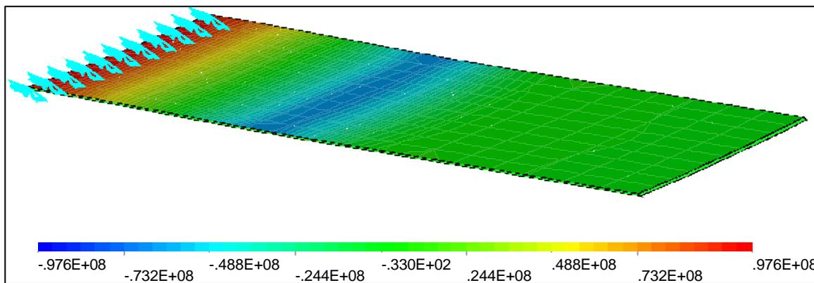
Fig. 7: Stress distribution in the membrane when contacted with an electrode (Units are Pa)
