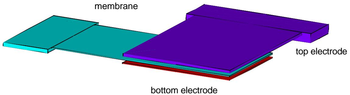
Fig. 6: Schematic view of the double anchor structure for mechanical simulation
