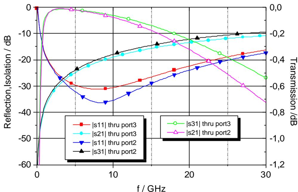
Fig.5: Simulation results of the SPDT build from double anchor switches (open/closed) position
