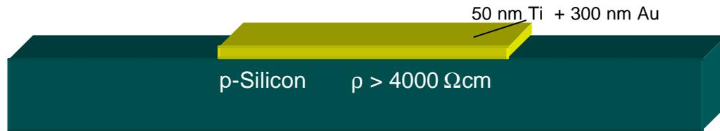
(1) Lower electrode (underpass – metallization): 50 nm Ti, 300 nm Au
