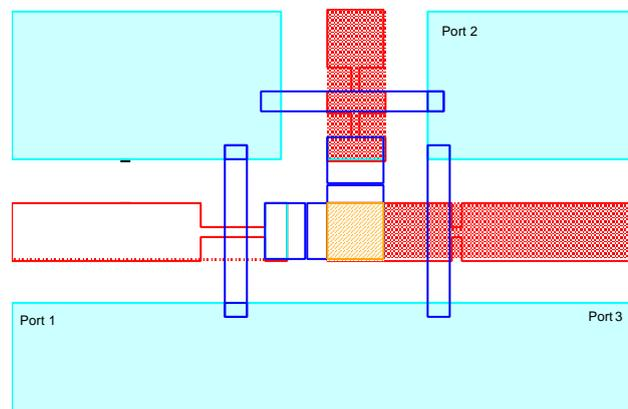
Fig.4 Schematic / layout view of the double anchor switch in SPDT operation
