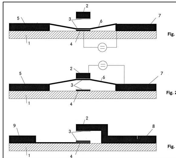
Fig. 2: Schematic concept of a so called "double anchor switch"
