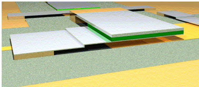
Fig. 3: Schematic concept of an STDT switch by using a double anchor switch
