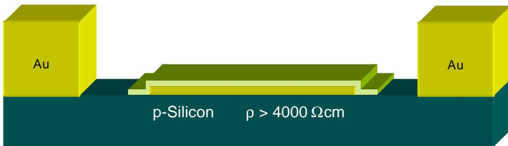
(3) Definition of the transmission lines: 50 nm Ti, 2500 nm Au
