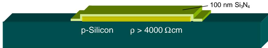
(2) Isolation layer for lower electrode: 100 nm  $\text{Si}_3\text{N}_4$
