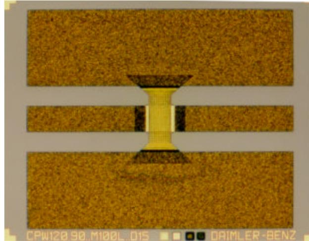
Fig. 9: Micrograph (layout) of a capacitive RF switch chip
