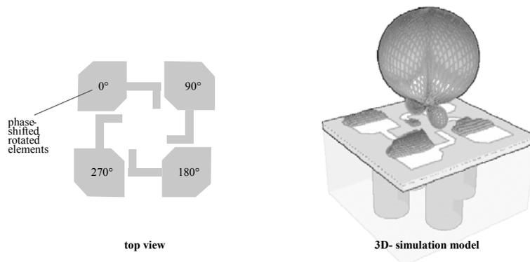
Fig. 4: Sequential rotated elements.
