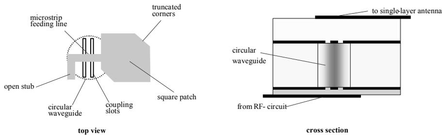
Fig. 3: Patch element with truncated corners and waveguide interface.
