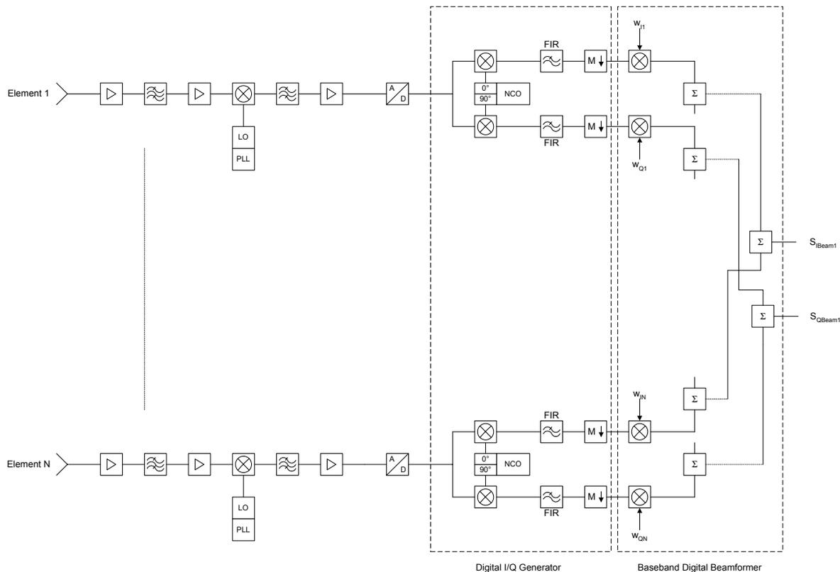
Fig. 2: DBF concept with digital I/Q generation.
