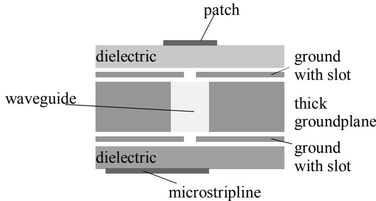
Fig. 5: Cross-section of single antenna element.
