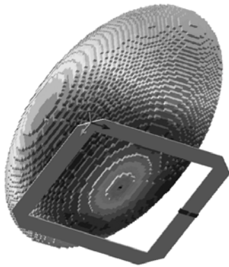
Fig. 8: Current density results in the ellipsoid model and model of an RFID coil.
