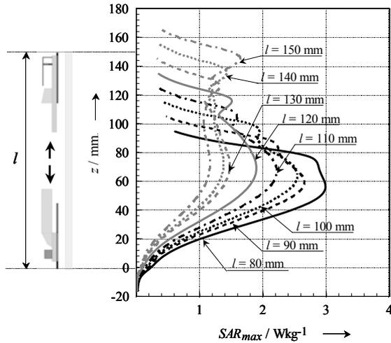
Fig. 4:  $SAR_{max}$  on the surface of a flat phantom for different models of a mobile phone: C-Patch antenna;  $f = 925$  MHz;  $P_{in} = 33$  dBm.
