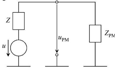
Fig. 3: Equivalent circuit for voltage transformation
