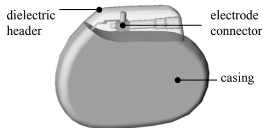
Fig. 1: Numerical model of a unipolar pacemaker
