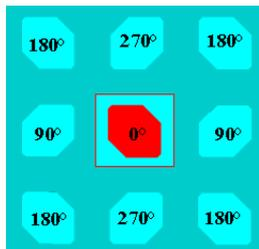
Figure 3: Basic coupling model (active patch = red).
