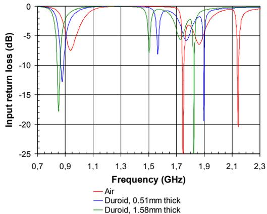
Fig. 4: Simulated input return loss of the quadband antenna on different substrates
