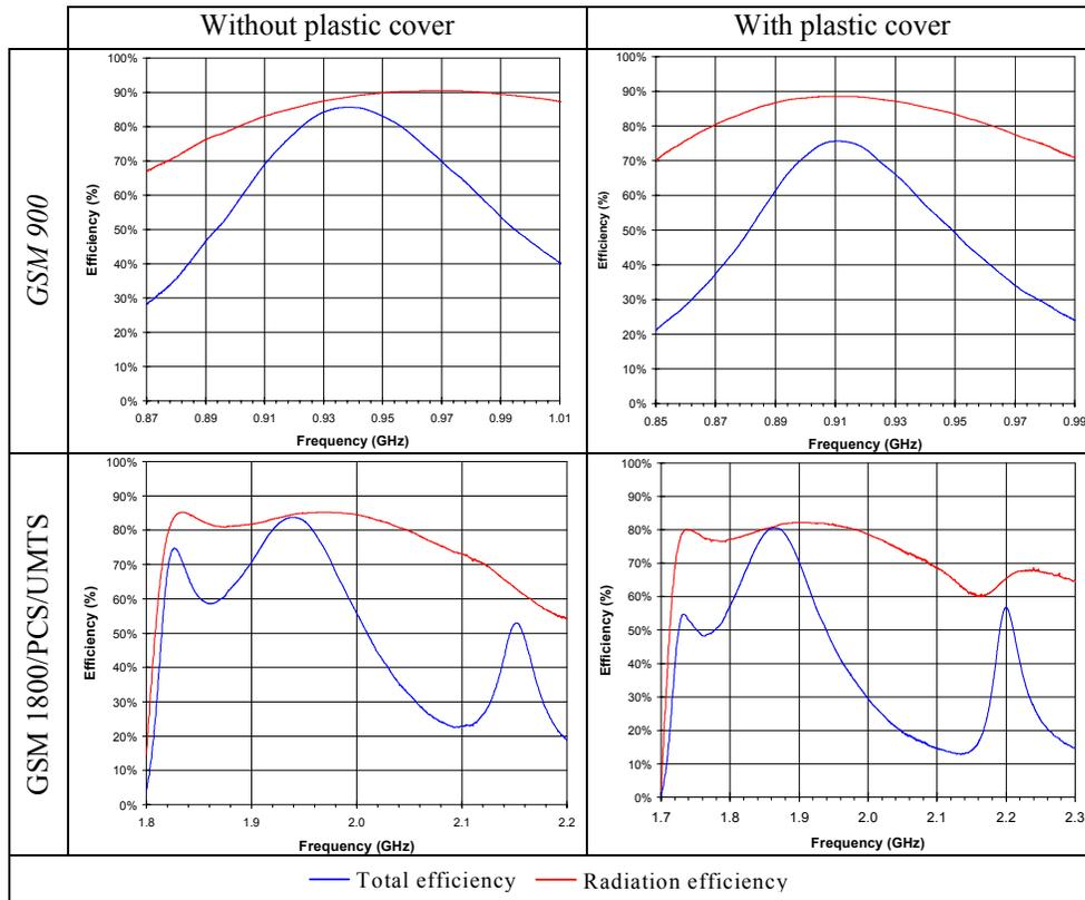
Fig. 6: Antenna efficiency, with and without plastic cover.
