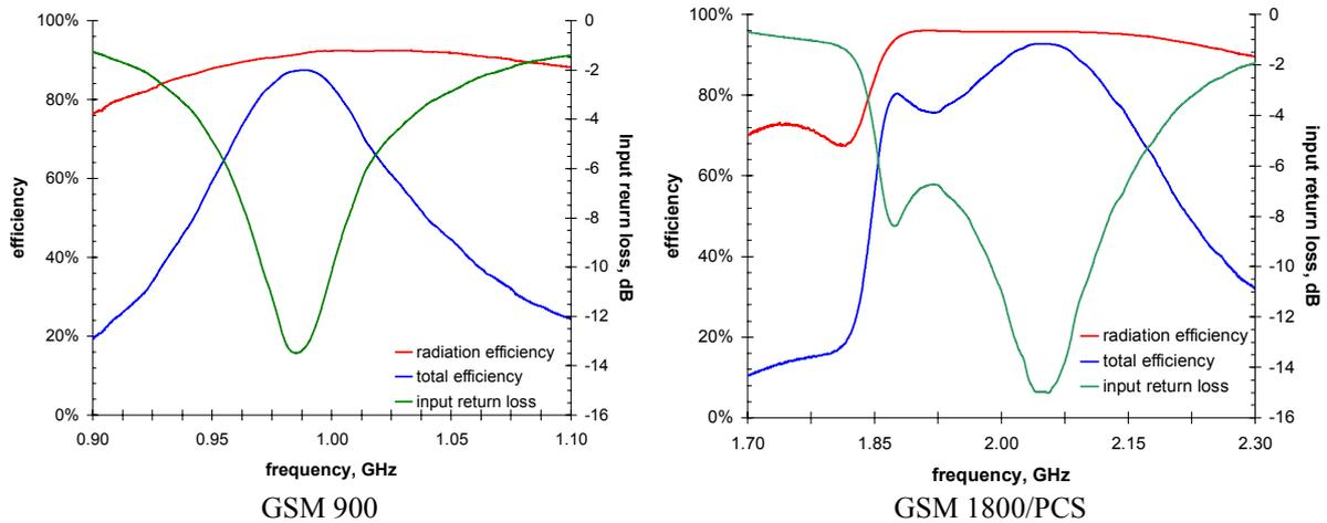
Figure 5: Antenna efficiency versus input return loss of the triple band antenna.
