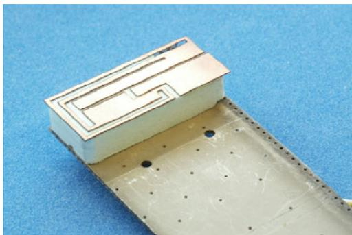
Figure 6: Quadband antenna.
