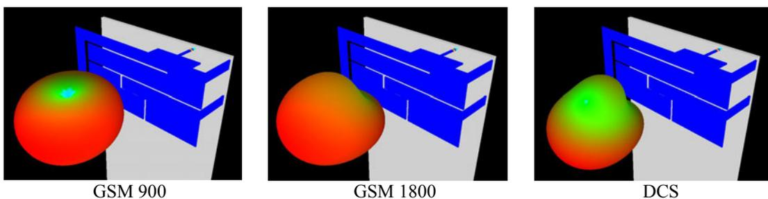
Figure 4: Radiation patterns of the triple band antenna.
