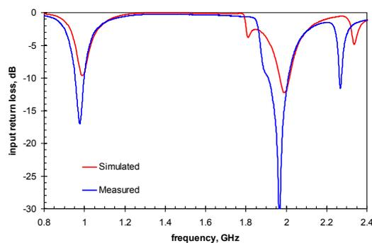
Figure 7: Input return loss of the quadband antenna.
