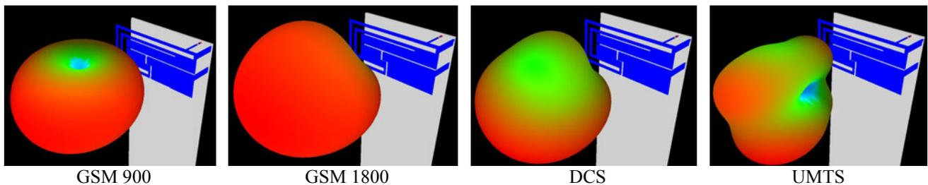
Figure 8: Radiation patterns of the quadband antenna.
