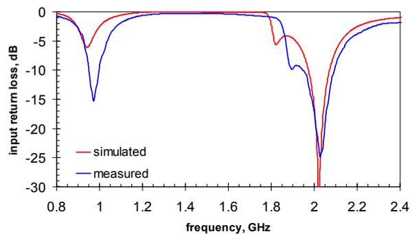
Figure 3: Input return loss of the triple-band antenna.
