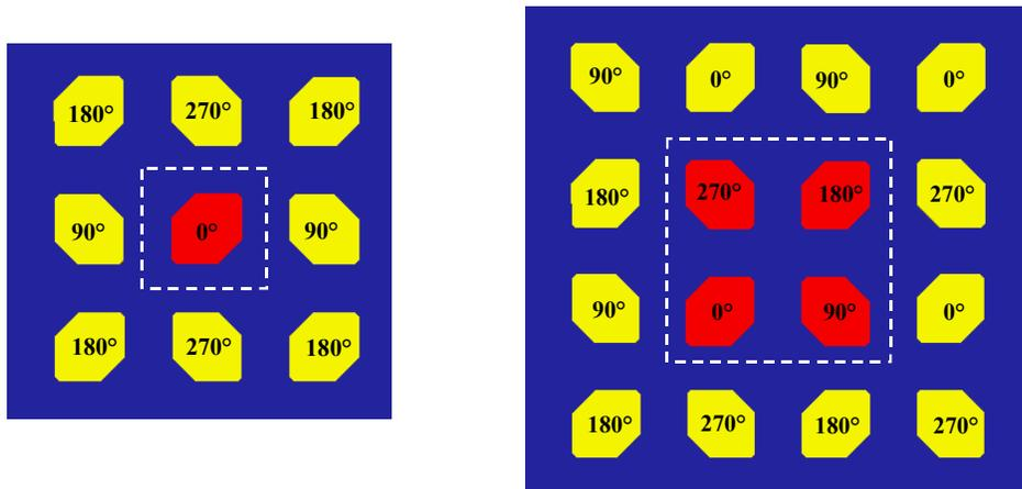
Figure 3. Coupling: general first order model (a), extended sequential rotated model (b), active patches in red.
