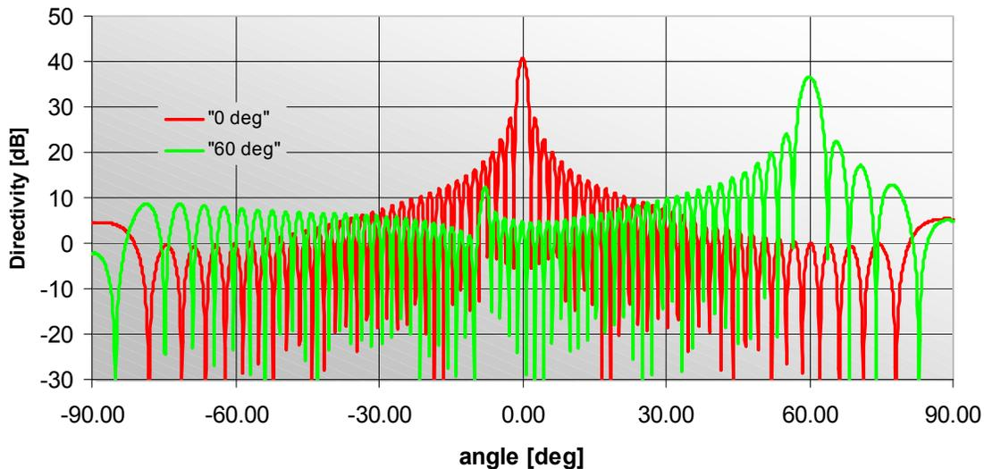
Figure 5b. Co-polar patterns of the phased array (64x64 elements), scan angles 0° and 60°, cardinal plane, with coupling.
