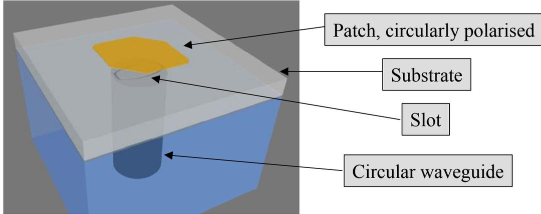
**Figure 1. Overview of the basic antenna element.**
