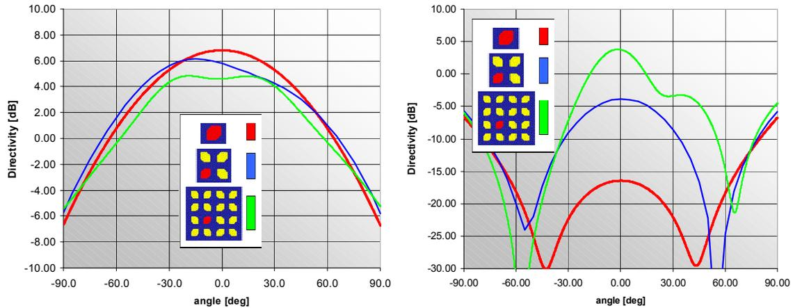
Figure 4. Co- (left) and cross-polar (right) patterns for different patch configurations, cardinal plane.
