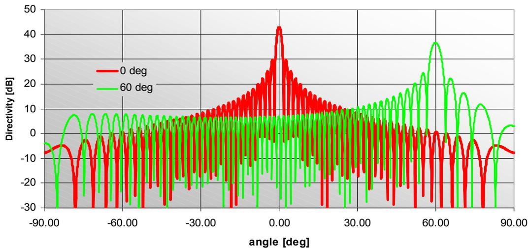
Figure 5a. Co-polar patterns of the phased array (64x64 elements), scan angles  $0^\circ$  and  $60^\circ$ , cardinal plane, without coupling.
