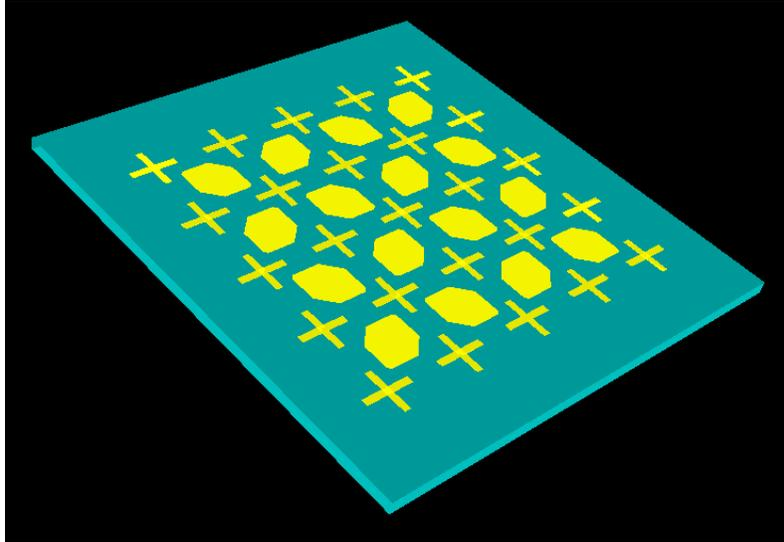
Figure 7. A possible improved layout for counteracting coupling.
