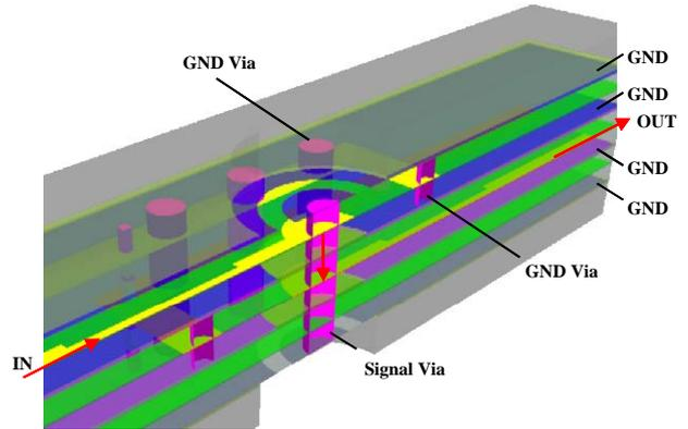
Fig. 5. 3D view into inter-layer transition
