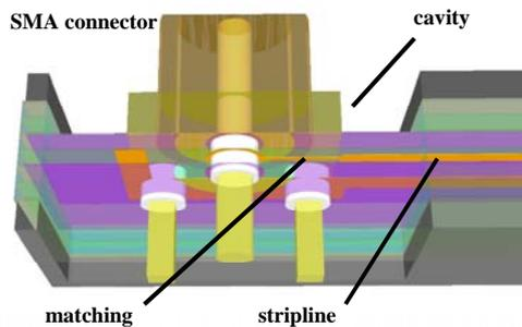
Fig. 7. 3D view into transition to SMA connector
