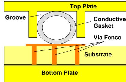
Fig. 3. Schematic of assembled "wall"
