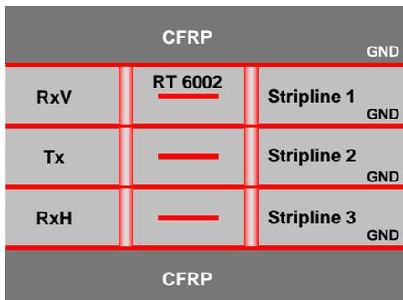
Fig. 4. Cross view of multilayer board
