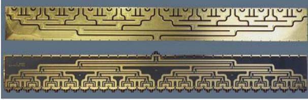
Fig. 1. Photograph of the 1:32 divider: housing, substrate and top cover
