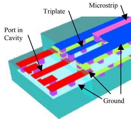
Fig. 15. Transition with shielding structures to minimize cross-talk: Microstrip  $\leftrightarrow$  Stripline  $\leftrightarrow$  Port in cavity
