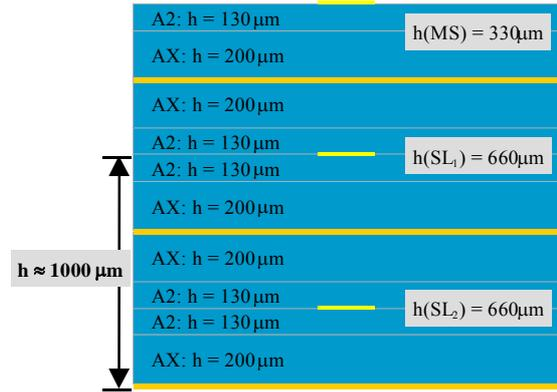
Fig. 11. Cross section of the divider module (material: Dupont 951,  $\epsilon_r = 7.8$ )
