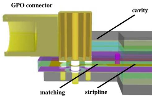
Fig. 6. 3D view into transition to GPO connector
