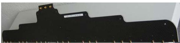
Fig. 8. Photograph of Elevation Feed Network
