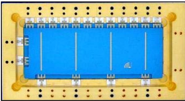
Fig. 10. Photo of divider module utilizing multilayer LTCC in a gold-plated DISPAL housing
