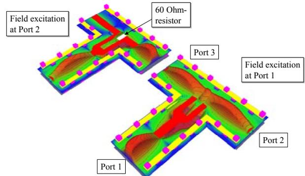
Fig. 12. Wilkinson divider in LTCC with electric field
