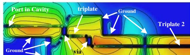
Fig. 16. Simulated electrical field in transition: Stripline  $SL_2$   $30\Omega \leftrightarrow$  Stripline  $\leftrightarrow$  Port in cavity
