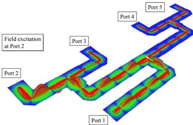
Fig. 13. (1 : 4) distribution network with electric field
