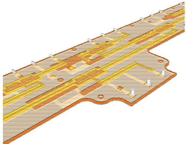
Fig. 9. Layout view of inner divider network structure
