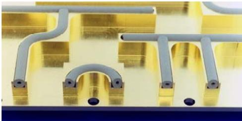
Fig. 2. Photo of the cover with grooves and gaskets
