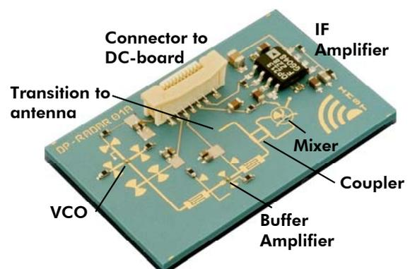
Figure 1: Frontend module on multilayer LTCC.
