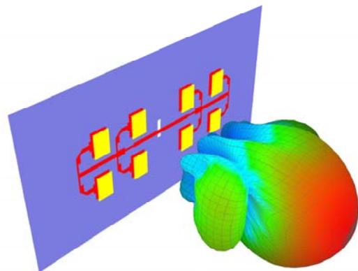
**Figure 4: Far-Field pattern of  $2 \times 4$  patch array.**
