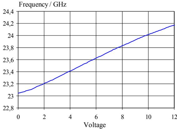
**Figure 2: VCO frequency as a function of control voltage.**
