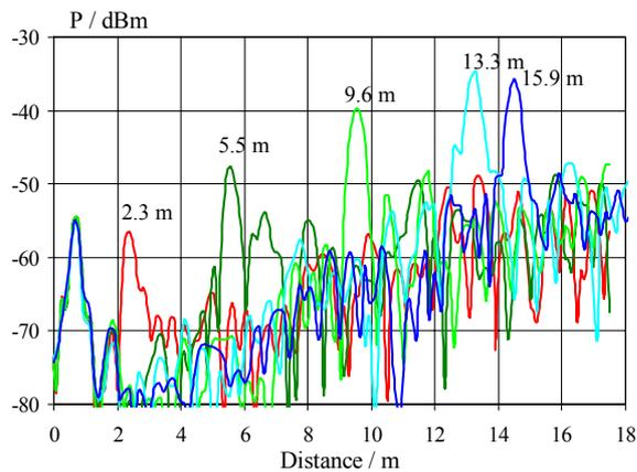
**Figure 8: Measured distances to cars on a street (b = 800 MHz).**
