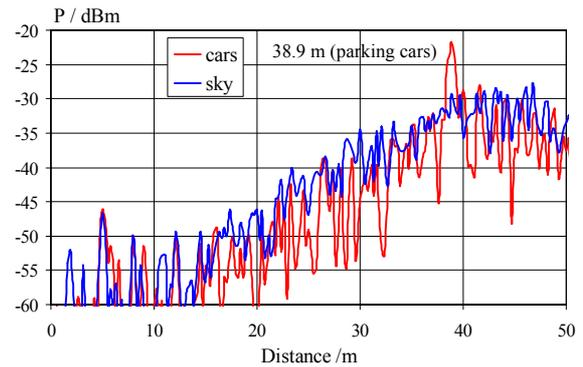
**Figure 7: Measured distances to parking cars.**
