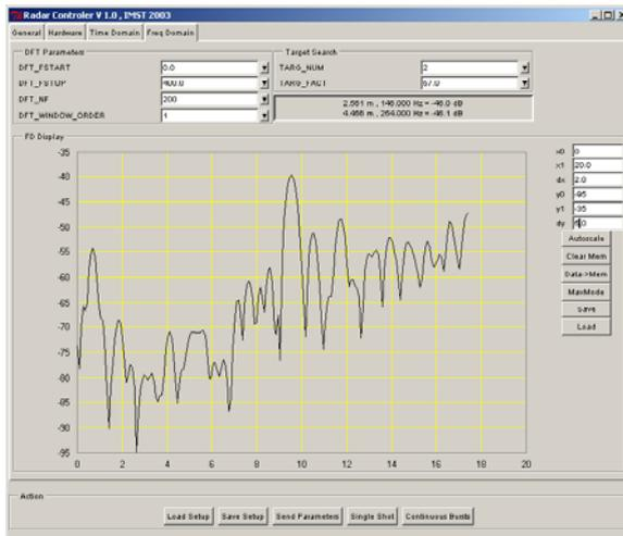
**Figure 6: Frequency domain settings and plot of evaluation software with graphical user interface.**
