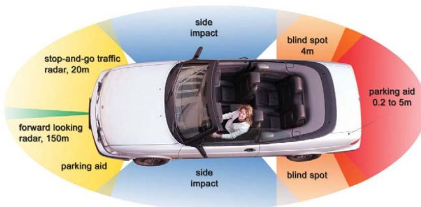
**Figure 10: Applications for automotive sensors.**
