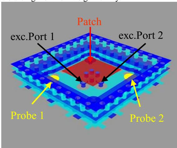
**Fig. 3: Patch antenna iso view.**
