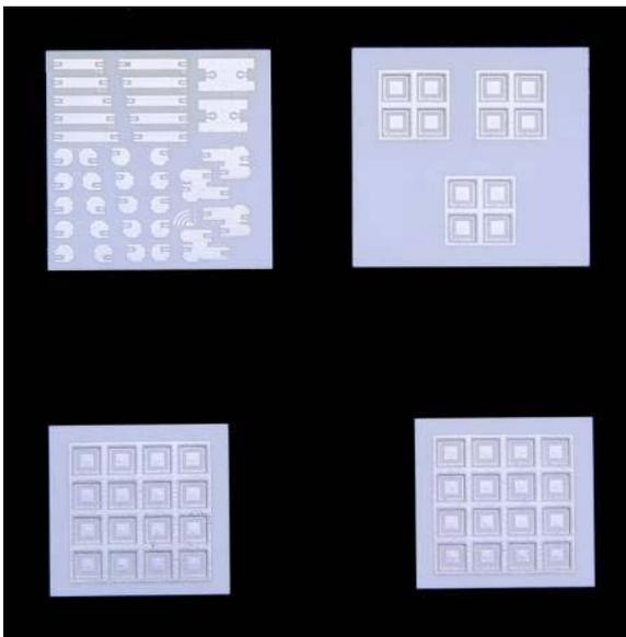
**Fig. 7 LTCC Test Tile**
