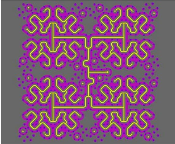
**Fig. 6: Whole calibration network for the 4x4 array.**
