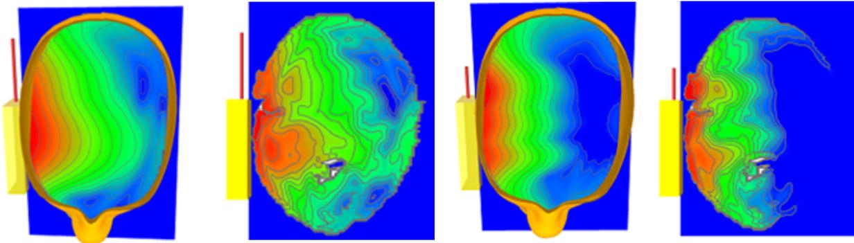
a) SAM phantom:  $\max(\text{SAR}_{1g}) = 7.5 \text{ W/kg}$ . b) Visible Human:  $\max(\text{SAR}_{1g}) = 5.4 \text{ W/kg}$ . c) SAM phantom:  $\max(\text{SAR}_{1g}) = 8.96 \text{ W/kg}$ . d) Visible Human:  $\max(\text{SAR}_{1g}) = 7.65 \text{ W/kg}$ .
